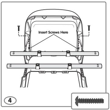
• Insert two #10 x 2,2 cm **black** screws through the footrest and into the seat bottom. Tighten the screws.
